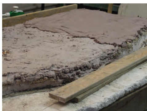
Fig. 12. The leveling of the backside of the mosaic was made by the lightweight lime-based mortar (Photo: Brigitta Maria Kürtösi)
