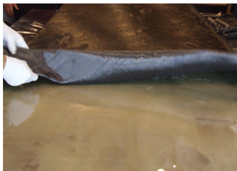
Fig. 9. The preparation of the new support with woven carbon fibre and 3PSP2 resin (Photo: Brigitta Maria Kürtösi)
